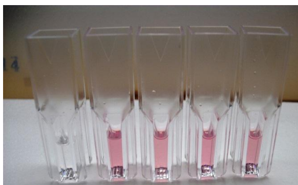
Figure 19 - Elastin samples in cuvettes for different concentration: Blank; Standard concentration 25 \mu\text{g} ; Sample of aorta; Sample of aorta with 6h isolation; Sample of aorta with 19h isolation.
