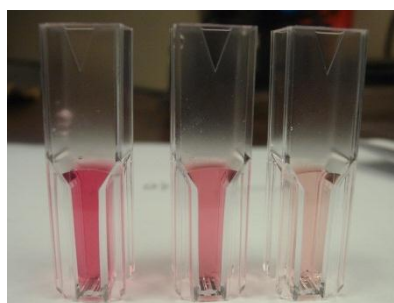
Figure 17 - Collagen standard in cuvettes for different concentration: left - 40 µg; middle - 25 µg; right - 7.5 µg.
