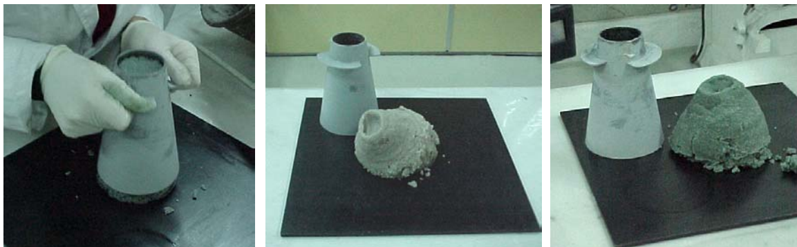
Fig. 4.1. Slump and flow tests of PM formulations: Cone removal (left) and typical slump shapes of epoxy and polyester PM formulations (center and right, respectively).
