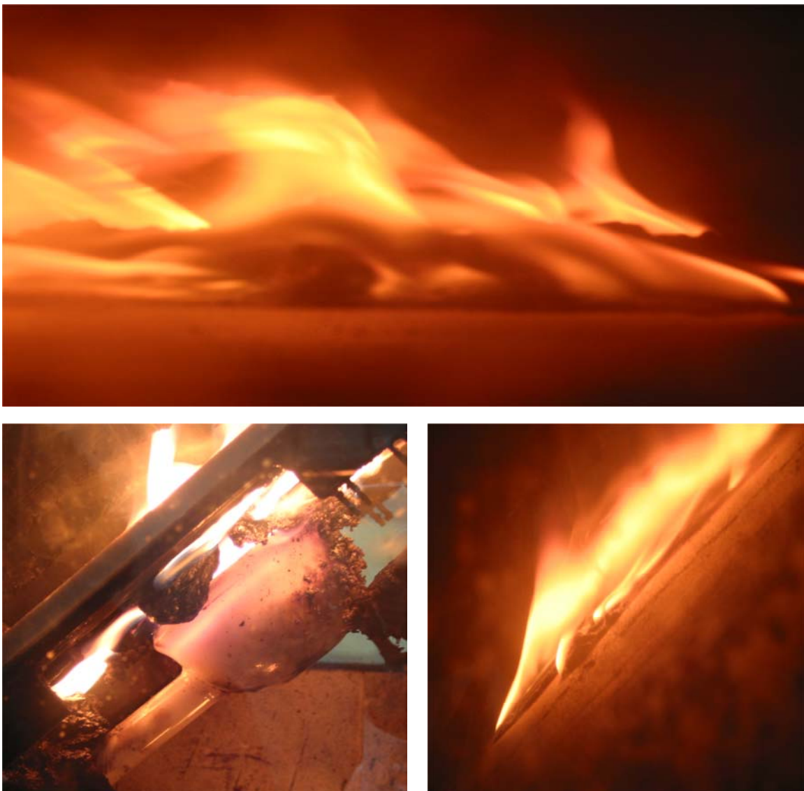
Fig. 6.10. Intumescent process occurring during fire radiation tests of epoxy PM specimens modified with APP flame retardant system.
