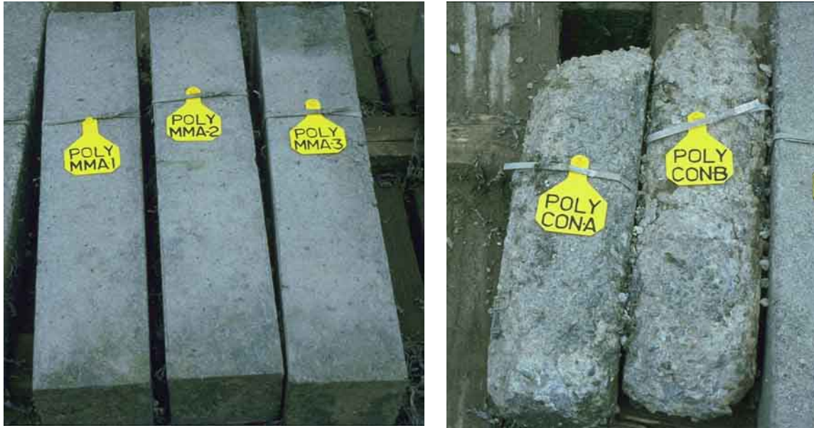
Fig. 2.4. Appearance of poly-methyl methacrylate PC specimens (left) and portland cement concrete specimens (right) after 20 years of outdoor exposure, according to investigation work reported by the U.S. Bureau of Reclamation (USBR 2006). Both types of beam specimens were installed near seawater and at half-tide elevation.
