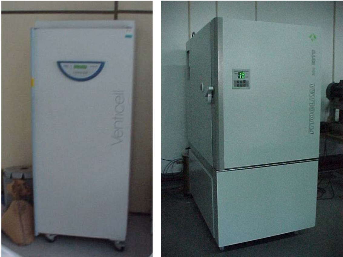
Fig. 3.5. Oven (at left) and climatic chamber (at right) used to dry the aggregates and for conditioning of PM specimens.
