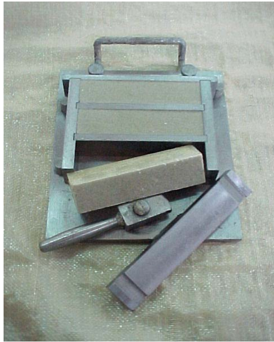
Fig. 3.3. Standard steel prismatic moulds for flexural testing purposes of polymer mortar specimens.
