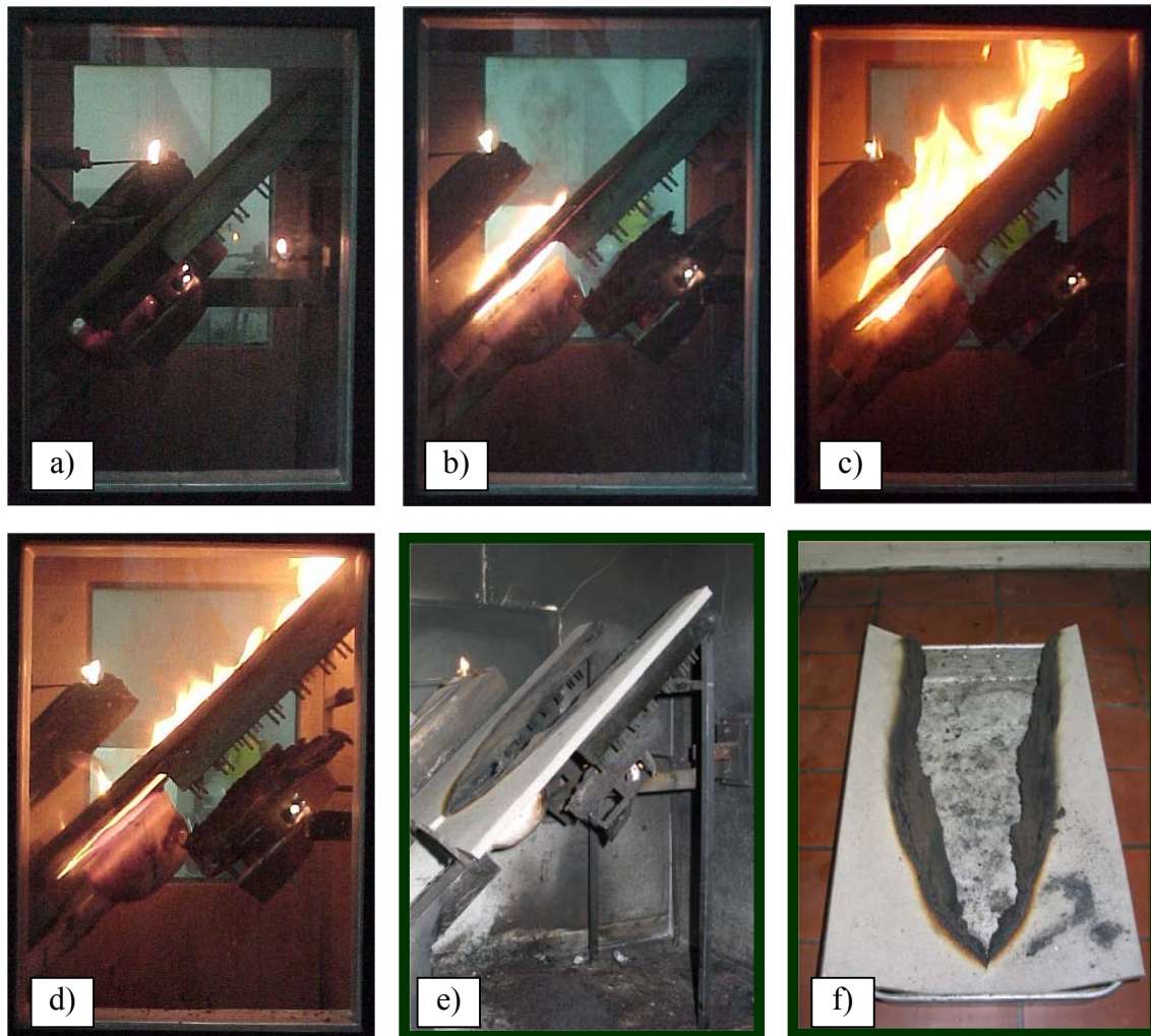
Fig. 6.9. Epiradiator test steps: a) Beginning of the test, with both gas burners already positioned against superior and inferior surfaces of test specimen; b) First effective inflammations on both faces of the specimen; c) Maximum combustion reaction, with flames reaching the maximum extent; d) Extinction of the flame on the inferior surface of the specimen; e) End of the test; f) Appearance of plain epoxy PM specimen after fire radiation test.
