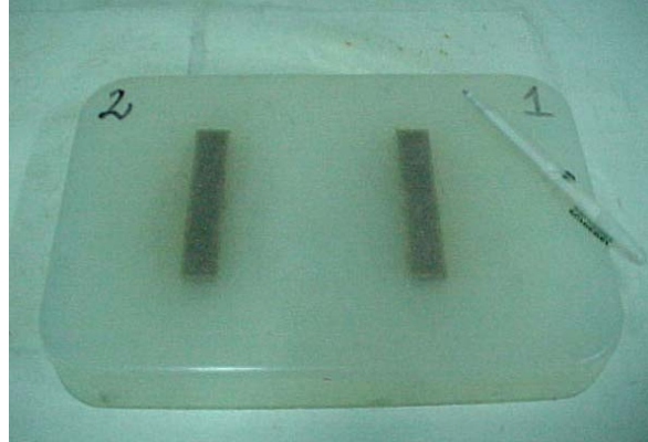
Fig. 4.3. Polyester PM specimens used for determination of final setting shrinkage.
