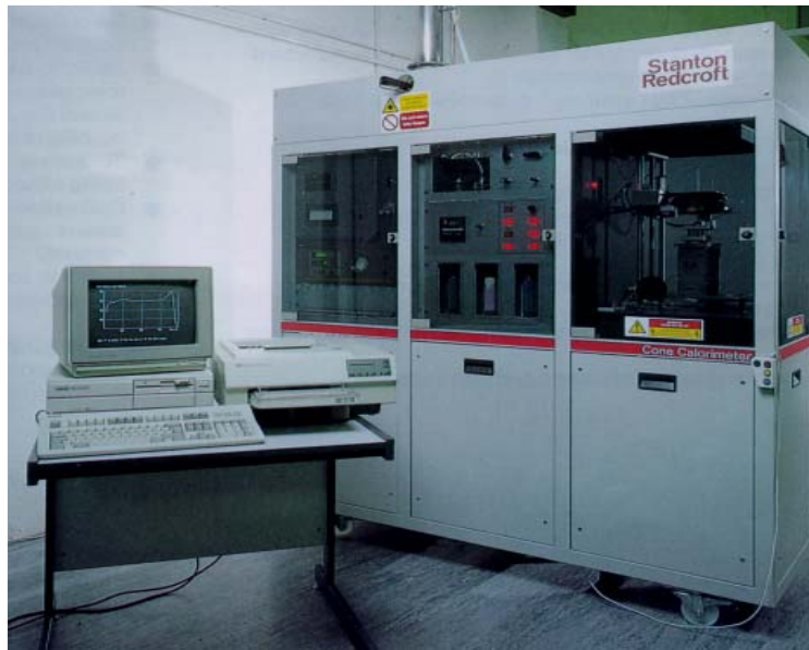
Fig. 6.1. Oxygen consumption calorimeter apparatus used to perform heat release tests.
