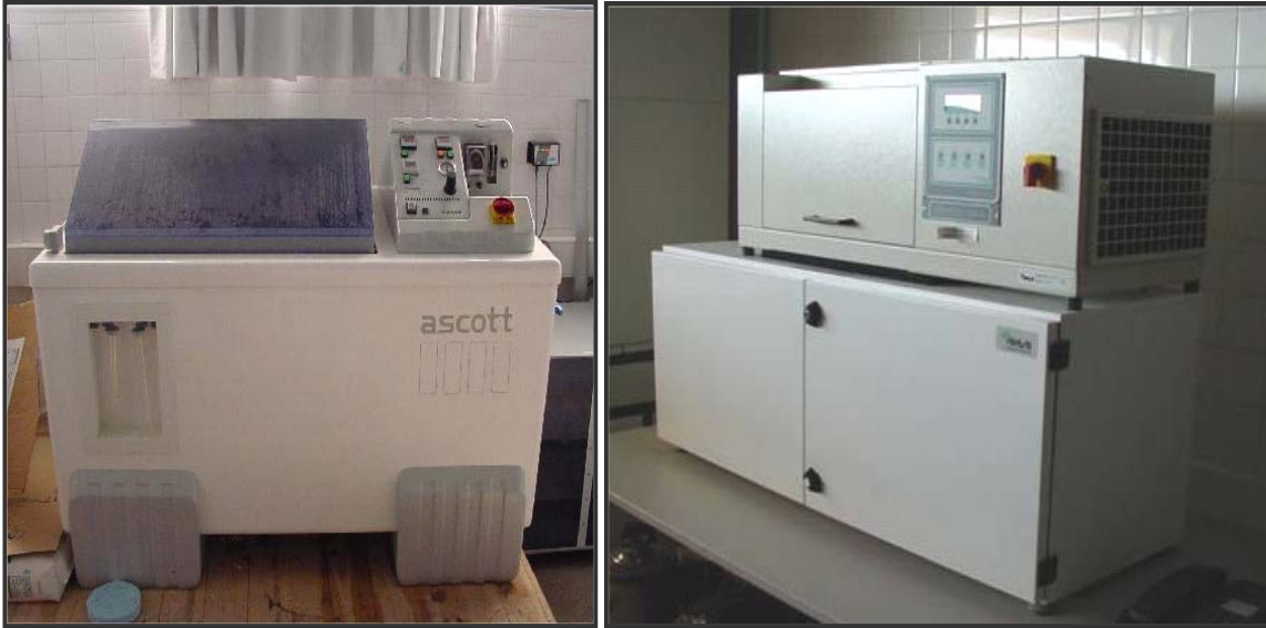
Fig. 5.23. Salt fog chamber (left) and arc xenon solar box (right) artificial weathering devices.
