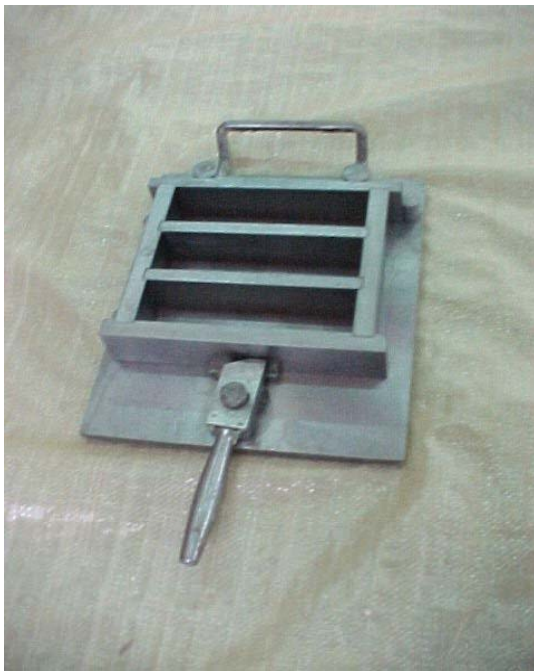
Fig. 3.3. Standard steel prismatic moulds for flexural testing purposes of polymer mortar specimens.
