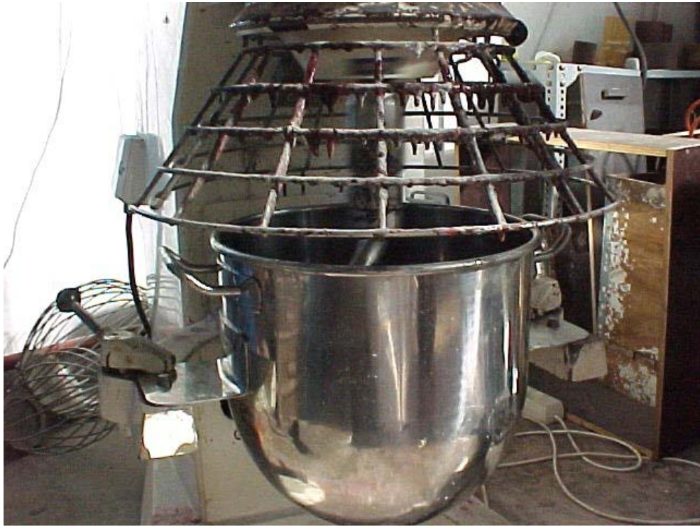
Fig. 3.2. Automatic batch mixer used to mix the polymeric resins with the aggregates.
