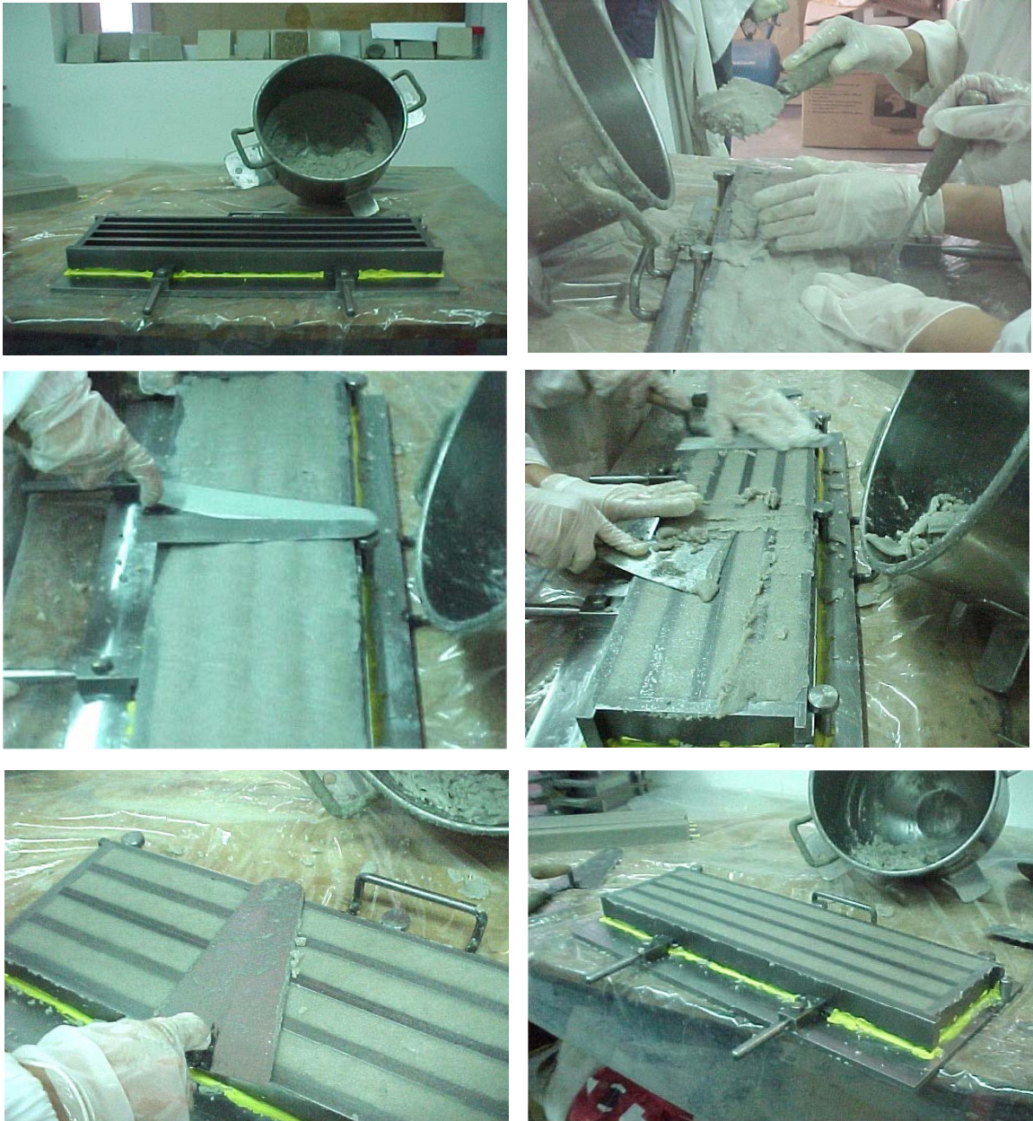
Fig. 3.4. Casting steps for moulding polymer mortar specimens.
