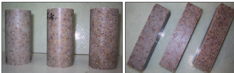
Fig. 1. Some examples of cylinder and prismatic specimens produced of cork-modified polymer mortars.
