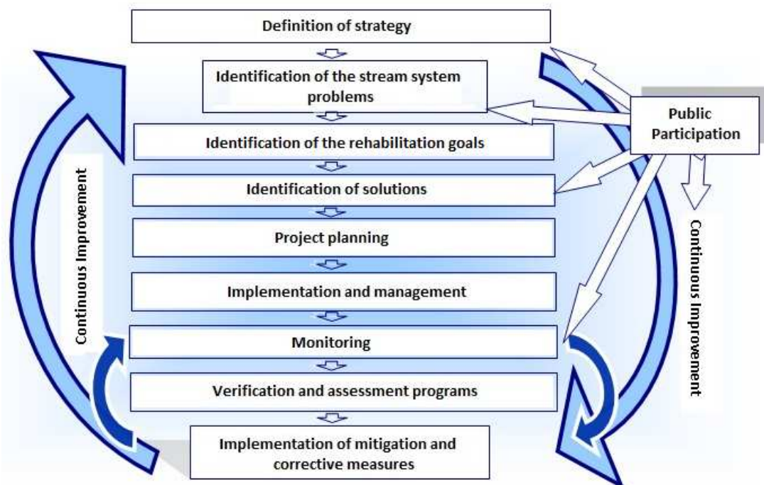
Fig.2: General scheme for the basic steps of stream rehabilitation (adapt. Teiga et al 2007)
