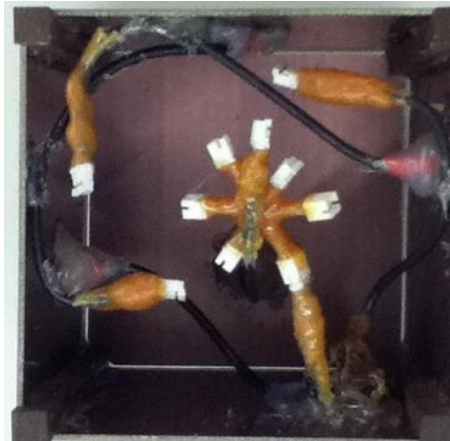
Figure 6.2: The Implemented Feed Scheme for the antenna array
