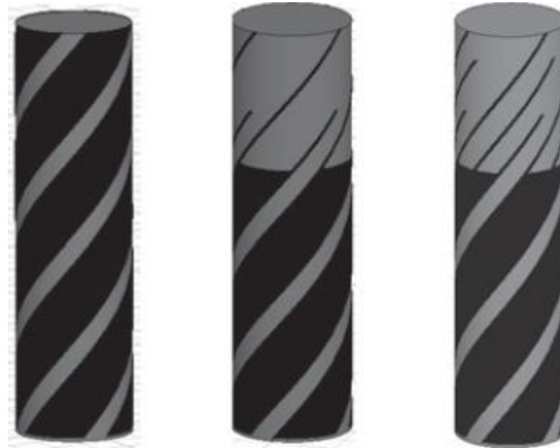
Figure 3.6: From the left to the right a scheme of a single, double and triple frequency band Printed Quadrifilar Helical Antenna [8]
