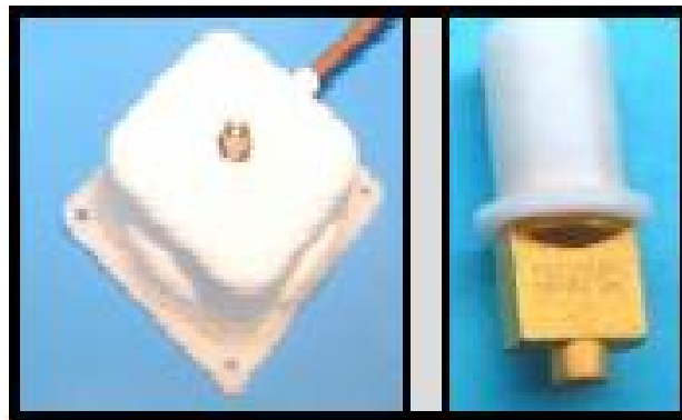
Figure 3.5: Example of a Patch Antenna on the left and of a Quadrifilar Helix Antenna on the right [7]
