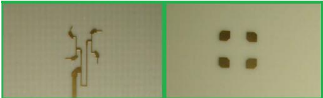
Figure 3.27: 60GHz Square Patch Antenna Array and its Feeding Network [18]
