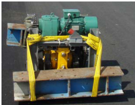
Figure 3.56 – Excitation device developed by CSTB with two steel profiles to increase its mass, and one of the measured free decays.
