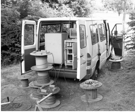
Figure 3.1 – Equipment for ambient vibration tests based on a central acquisition system (Wenzel and Pichler 2005).
