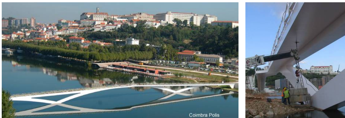
Figure 3.51 – Pedro e Inês Footbridge (general view and hanging of a mass for application of an impulse)
