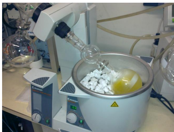
Figure. 8 Methanol recovering in a rotary evaporator.
