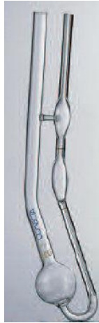
Figure. 10 Cannon-Fenske Viscosimeter with a total longitude of 250 mm.
