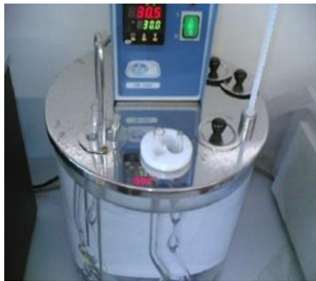
Figure. 11 Experimental apparatus – Thermostatic agitated bath with immersed viscosimeters.
