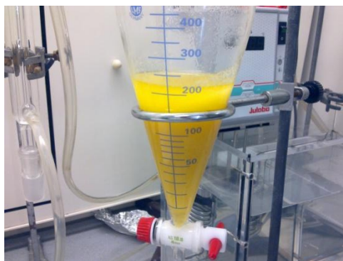
Figure. 7 Biodiesel and glycerol separation
