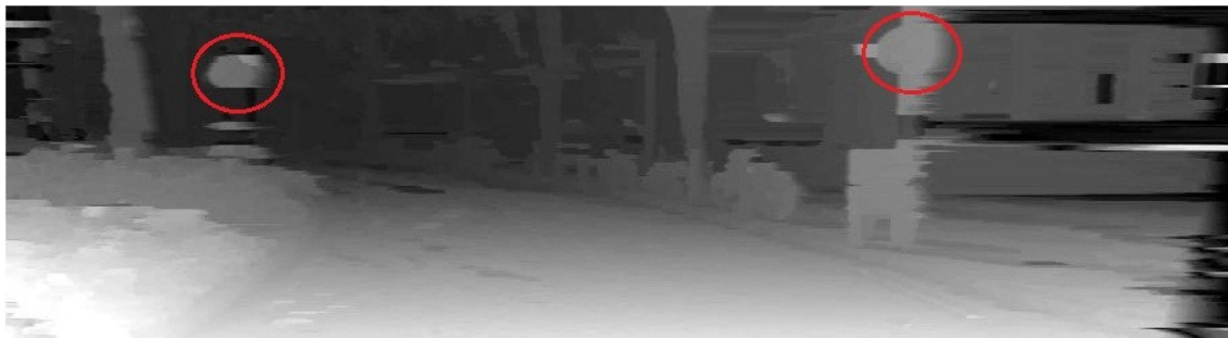
Figure 55 – Disparity map from the image shown in the Figure 54 with the two road signs circled with a red line
