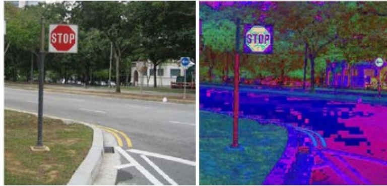
Figure 9 – RGB colour space and HSI colour space [19] (correspondently from the left image to the right)
