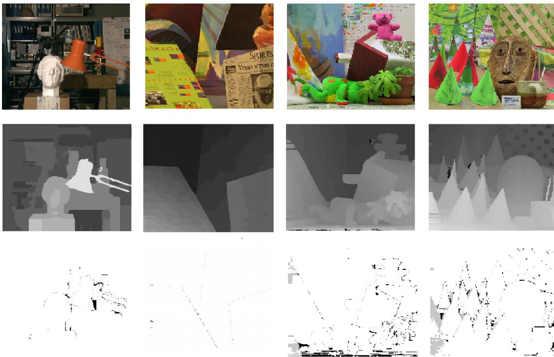
Figure 17 – Stereo matching results from the algorithm in [45]. From the top to the bottom is the original image, the correspondent disparity map and the error map with the bad pixels.
