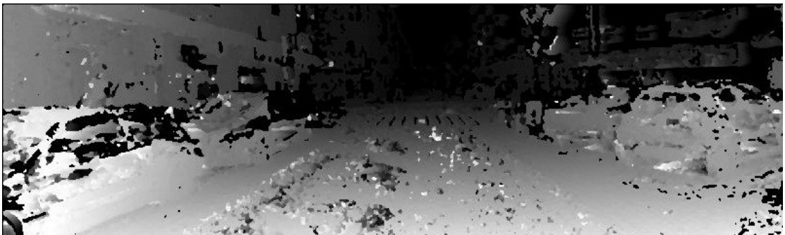
Figure 41 - Resulted disparity map of “Region” with the input parameters of 100 for disparity range and 5 for block matching window.
