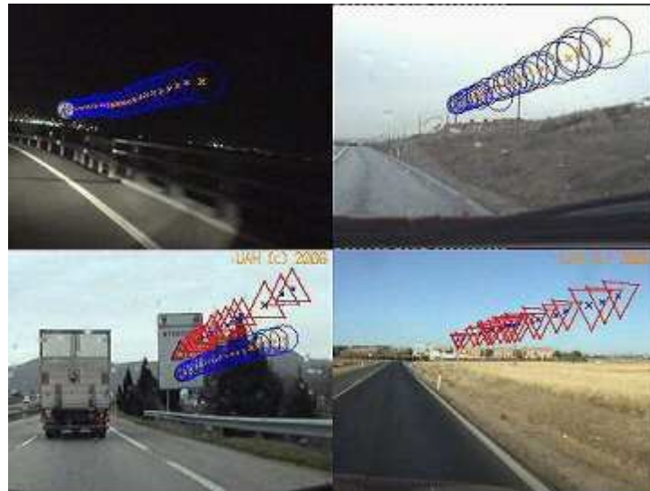
Figure 10 – Example of kalman filter usage in road sign tracking [20].
