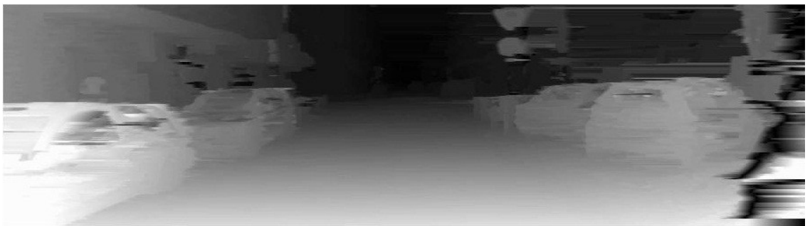
Figure 35 - Resulted disparity map of “Blockset” with the input parameters of 100 for disparity range and 5 for block matching window.
