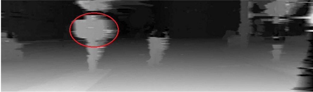
Figure 84 – Example of disparity image containing a vertical road sign circled by a red line.
