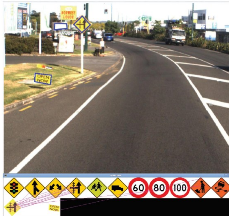
Figure 12 – Example of sign recognition using SIFT [25].
