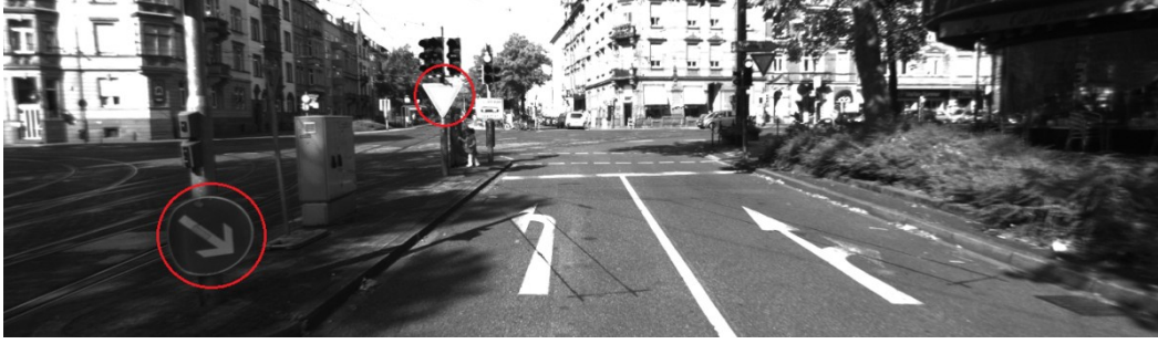
Figure 90 - Test image used as an example for the results of global localization of road signs. The image has two signs that are circled by a red line.
