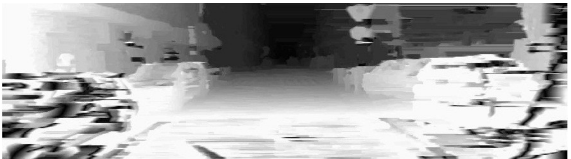
Figure 34 - Resulted disparity map of “Blockset” with the input parameters of 50 for disparity range and 7 for block matching window.
