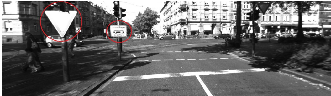
Figure 87 – Test image used as an example for the results of global localization of road signs. The image has two signs that are circled by a red line.
