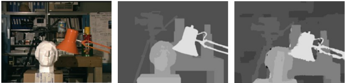
Figure 24 - Stereo matching result of [52]. From the left to the right, there is test image, the correspondent ground truth and the resulting disparity map.
