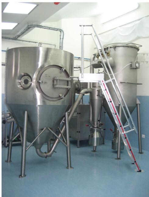
Figura 9 - Spray-Dryer Production Minor™, Gea Niro
