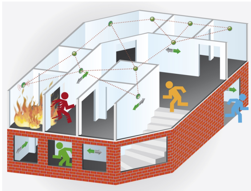
Figure 1.2: Pictogram of a evacuation system based on wireless sensors and guiding signs
