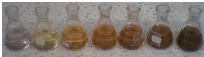
Figure III. 1.6 – Reactive blue 114 solutions after treatment with increasing ABTS concentrations (from left to the right).
