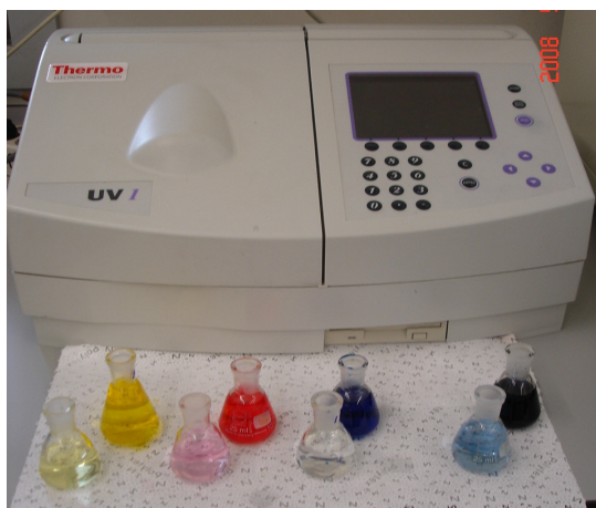
Figure III. 4.4 – Initial and treated solutions of RY15, RR239, RB114 and RB5, showing the decolourizations achieved.
