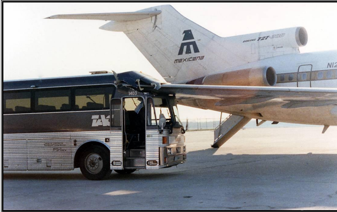
Figure 2-19 Example of ground crew error in ramp operation Source: Elbert (1980)
