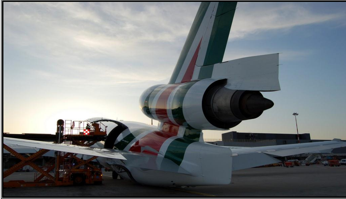
Figure 2-13 Example of Wrong Unloading/loading in Turnaround Process Source: Selman, (2004)
