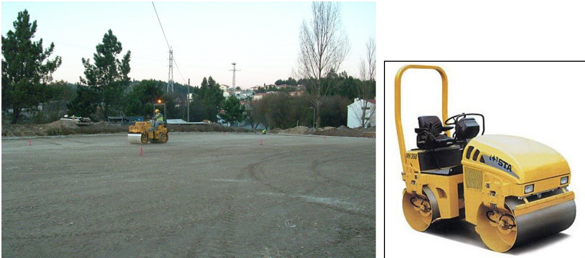
Fig.5.13 – Cilindro compactador ( http://www.logismarket.pt/lamaquina/cilindro-tandem/1274786301-920865001-p.html ).
