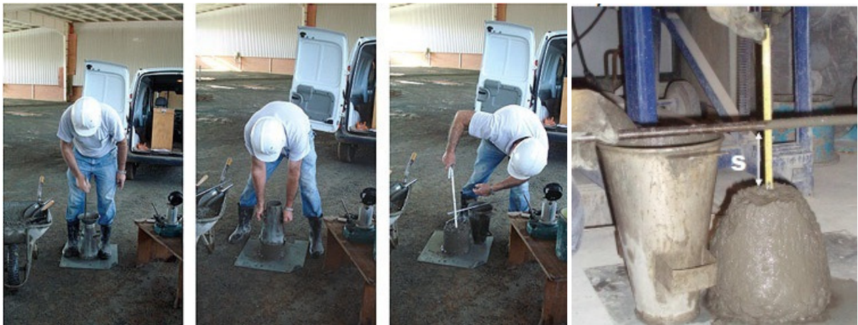
Fig.2.4 – Slump Test ( http://www.revistatechne.com.br/engenharia-civil/163/artigo189448-1.asp ).
