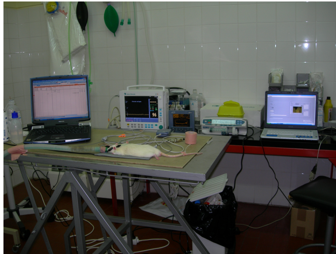
Figure 3.15: First Version of ASYS with BIS and infusion pump ASENSA in clinical trial with a mice.
