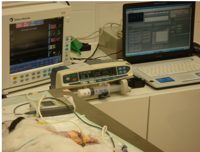
Figure 3.22: ASYS with controlled pump in clinical trial with rabbits - UTAD.
