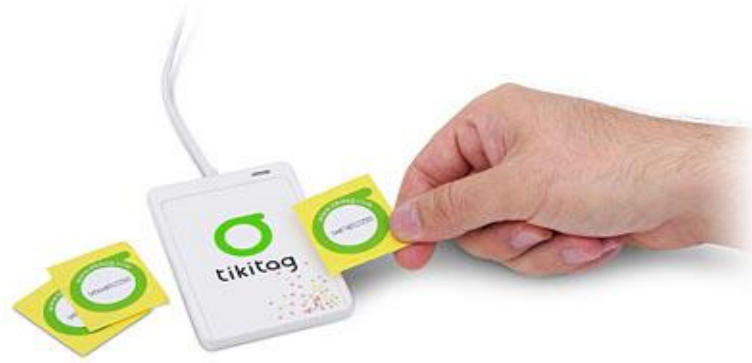
Figure 3.2- RFID passive tag and reader.
