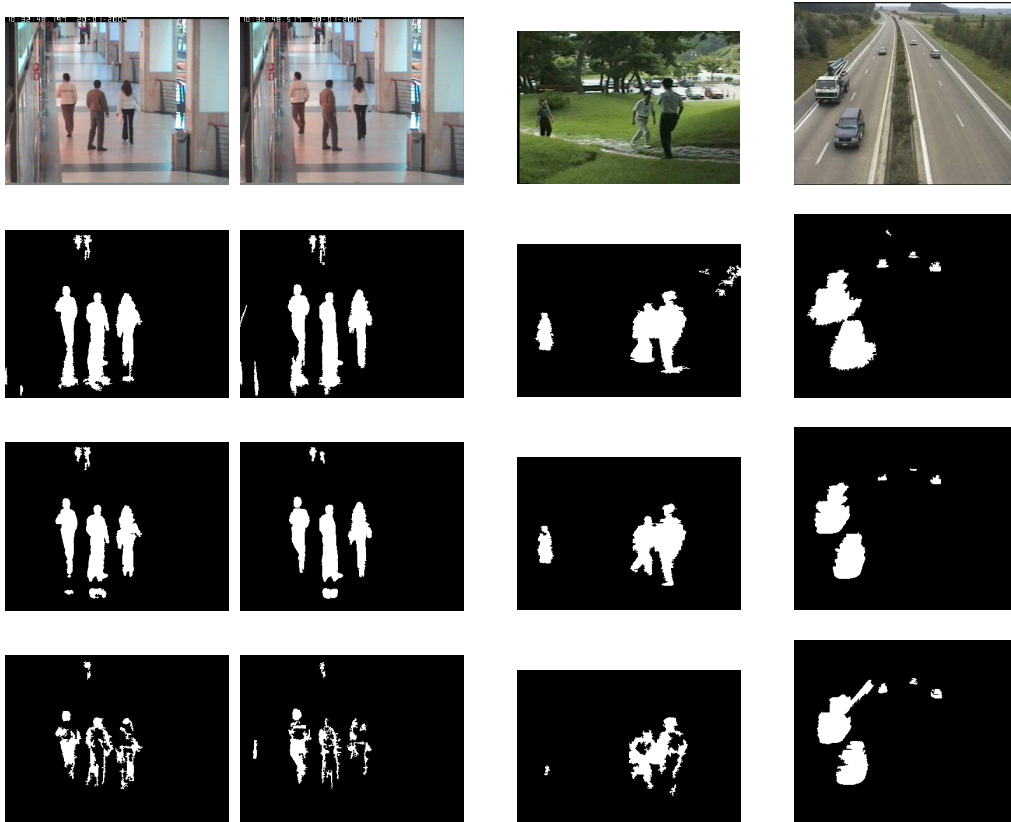
Figure 3.12: Segmentation masks obtained using different methods. The top row shows the original frame. The second row shows the results from the MoG implementation (Lee, 2005). The third row shows the results obtained with CMoG. Finally, the fourth row shows the results with CKDE.
