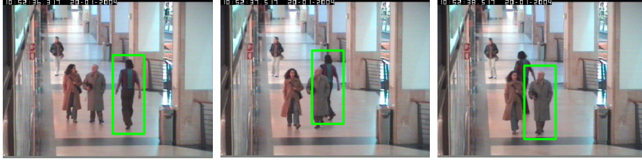
Figure 5.9: Common tracking error using a state-of-the-art particle filtering tracker. The tracker changes targets because the new target has a higher classifier score than the initial one. (Chateau et al., 2005)
