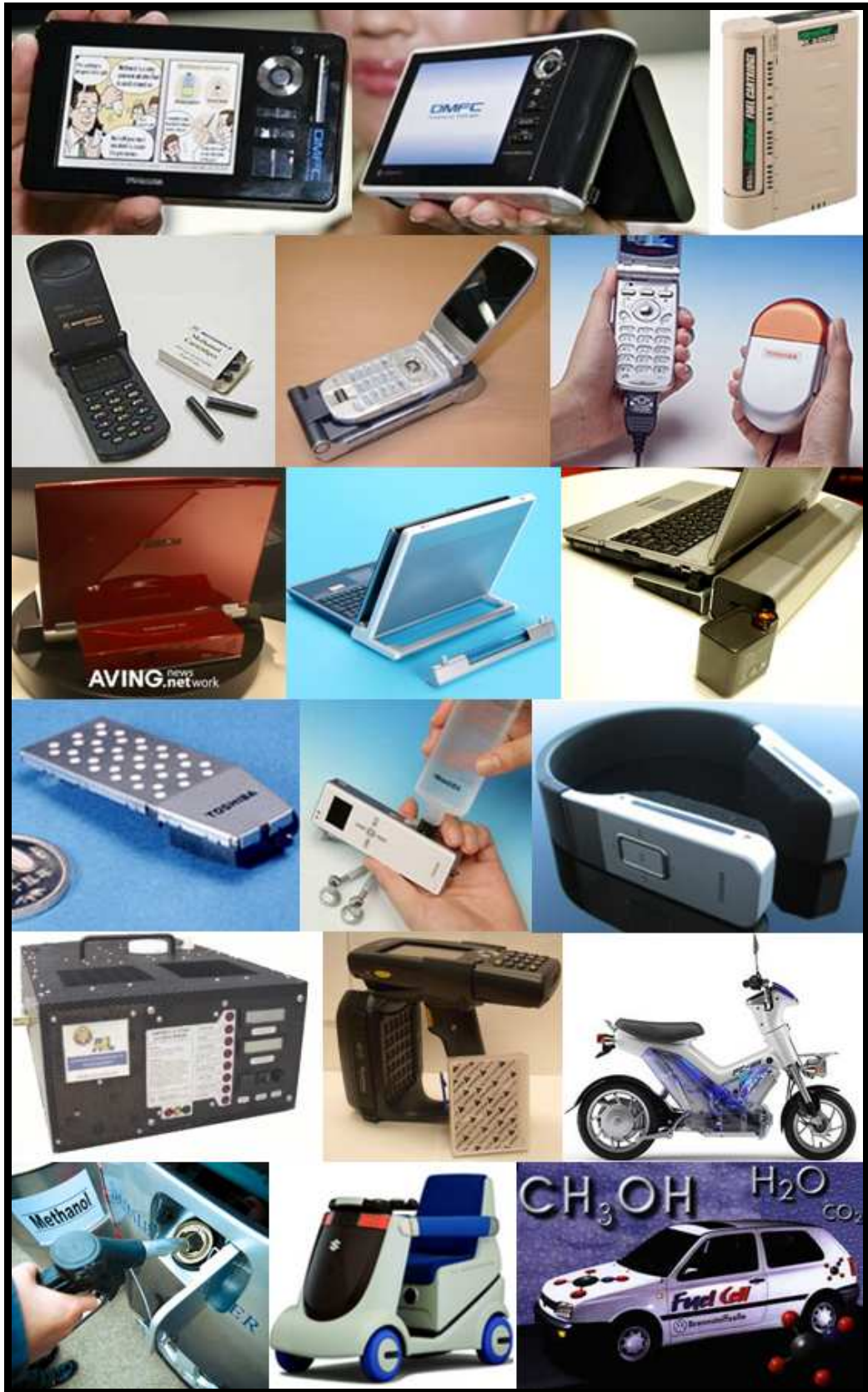
Figure 2.13 – Direct Methanol Fuel Cell applications (Courtesy Toshiba, Samsung, Motorola, Suzuki, Company's XX25, Yamaha, DaimlerChrysler, DoCoMo and Fujitsu, Intermec, Panasonic, Volkswagen).
