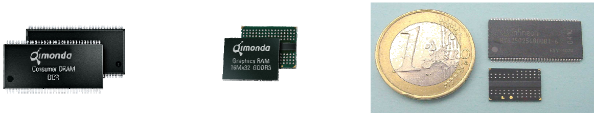
Figure 6 – TSOP (left side), BOC (center) components and their relative sizes (right side)
