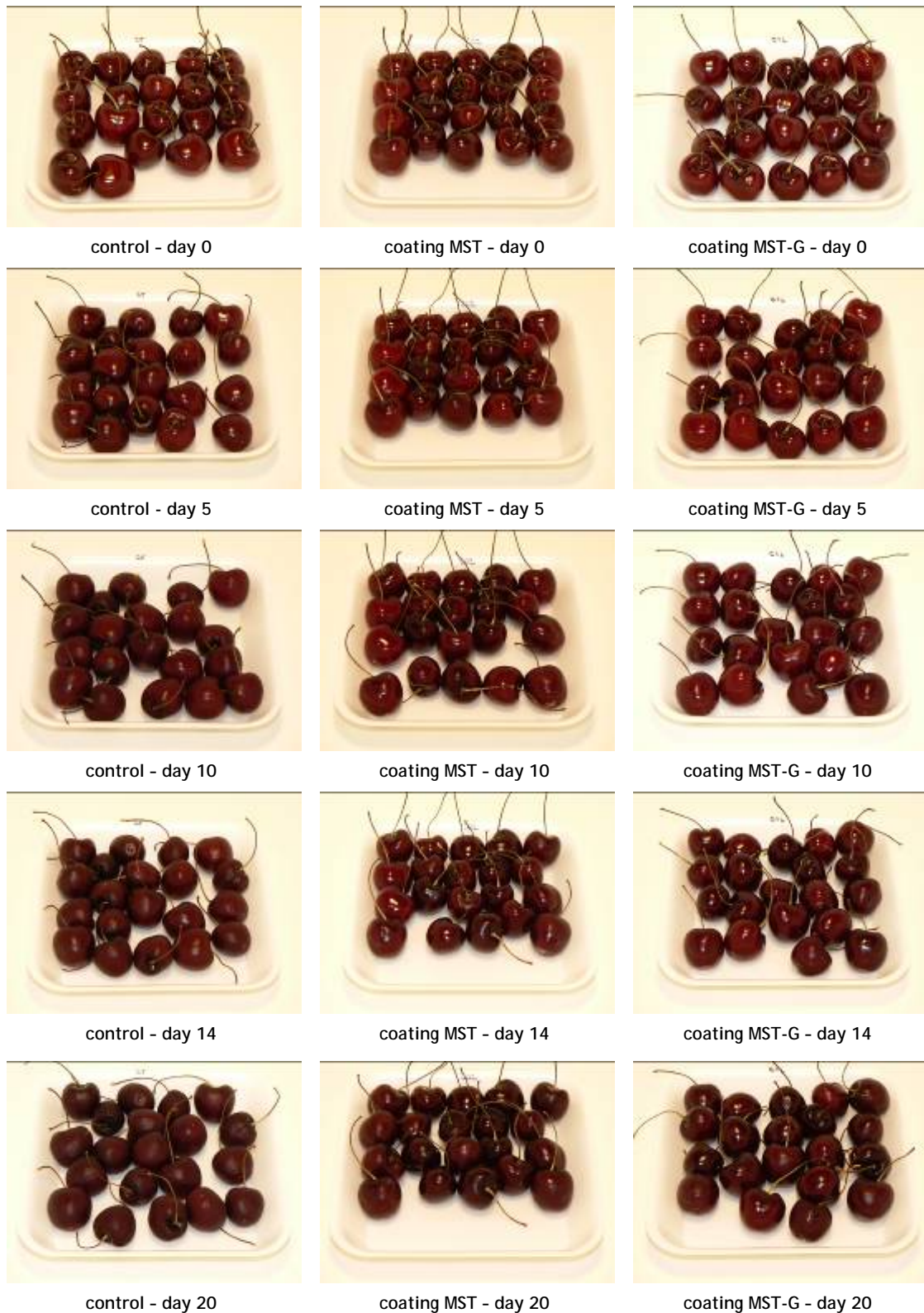
Figure 7.9 - Cherries not coated (control) and coated with \kappa/\iota -hybrid carrageenan (coating MST) and \kappa/\iota -hybrid carrageenan with the addition of glycerol (coating MST-G), at 0, 5, 10, 14 and 20 days of storage at 5 \pm 2^\circ\text{C} and 80-85% RH.
