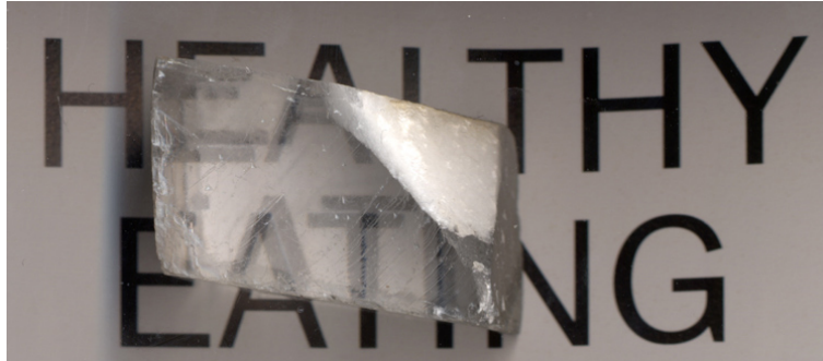
Fig. 2.1 A calcite crystal laid upon a paper with some letters showing birefringence effect [Image Released to the public domain by Adrian Pingstone in May 2003]
