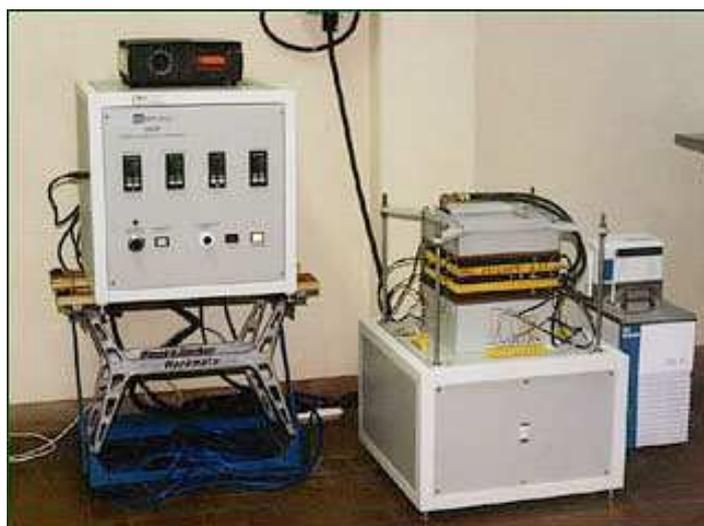
Figura 2.1 – HOLOMETRIX GHP-300 do LFC [13]
