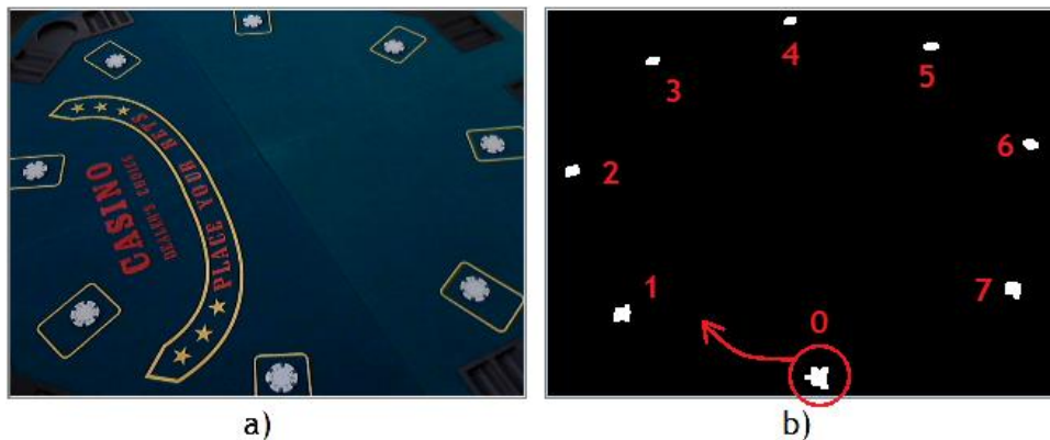
Fig. 6.1 - a) overview of the table with the white chips placed on the pre-defined squares for the cards; b) and the resulting image after colour segmentation and eroding+dilation
