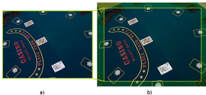
Fig. 4.4 - Region captured by the webcam in a fixed position, but set with different resolutions, where a) is set at 640x480 and b) is set at 800x600.
