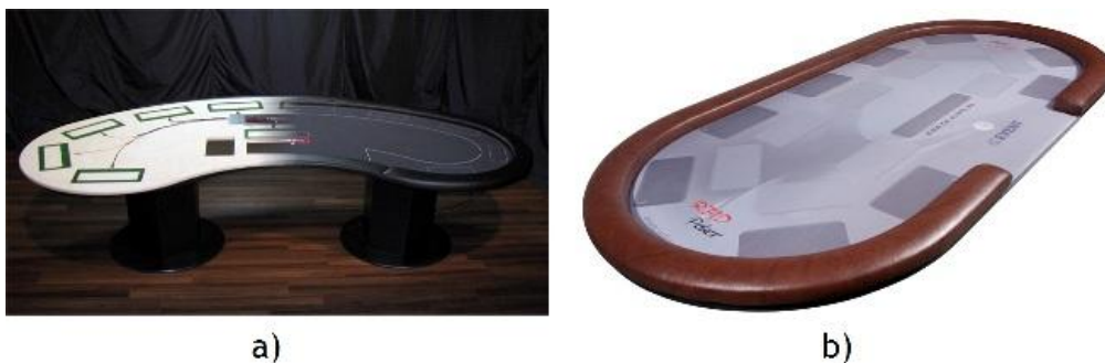
Fig. 3.2 - a) PokerTronic's table, where it is possible to see the RFID readers in the first half of the table; b) Flashlight Design Electronic System's poker table, the RFID readers can be spotted by the dark grey squares;
