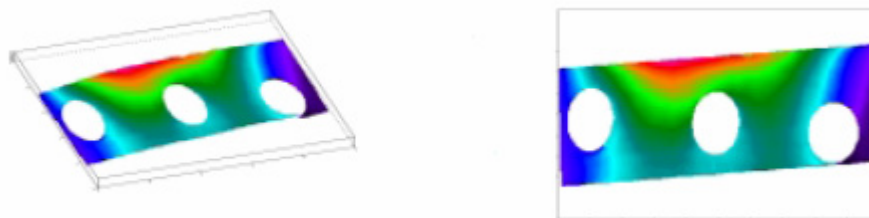
Figure 3.46 – Displacement field of the carbon/epoxy plate.
