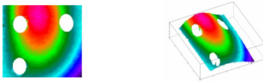
Figure 3.44 – Displacement field in the normal direction to heated plan of a glass/epoxy plate.
