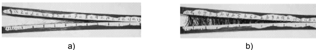
Figure 4.13 – Picture of a) 0^\circ/0^\circ and b) 0^\circ/90^\circ specimens after testing [154].
