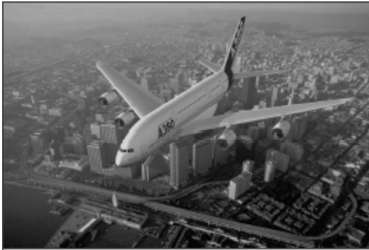
Figure 3.1 – The Airbus A380 – about 26 tons of carbon composite in each aircraft. Source: Reinforced Plastics.
