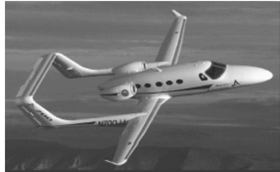
Figure 3.2 – Adam A700 all-composite personal jet. Source: Reinforced Plastics.
