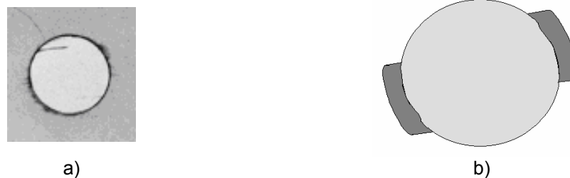
Figure 4.19 – Delamination area of a twist drill hole: a) radiography; b) finite element model.
