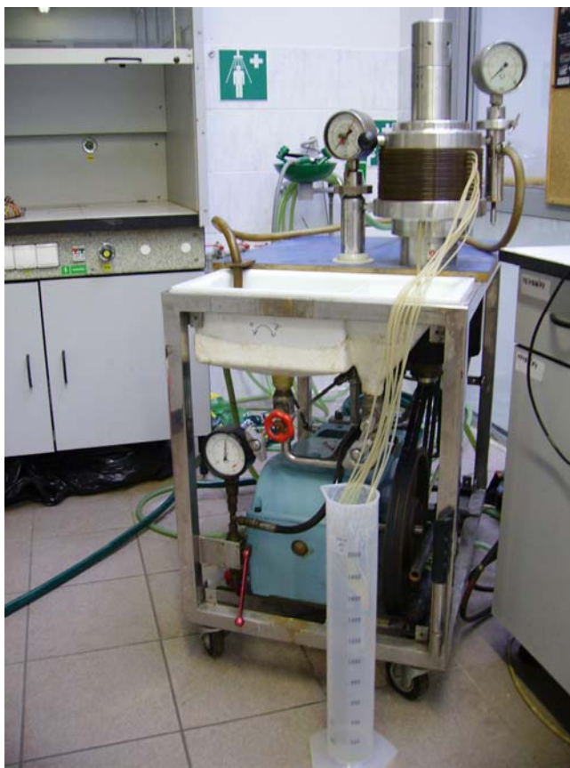
Figure 9: RO module - DSS Labstak M20
