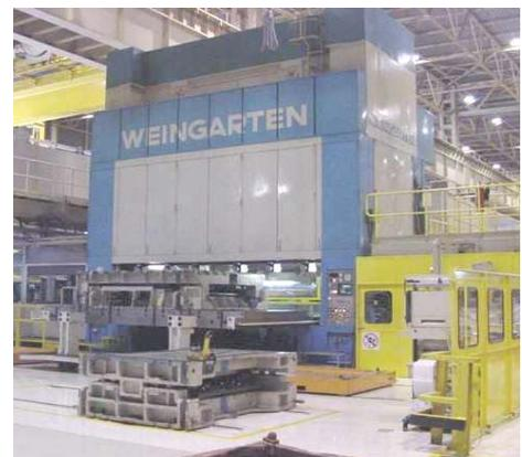
Figura 13 – Blanking Shear Line
