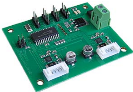
Figura 5.30: Driver Motor DC - Devantech MD25 Dual 12V 2.8A H-Bridge
