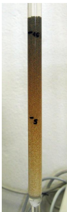
Figure 10: Image of the adsorption of Mo (V) onto Purolite D 4123 ®
