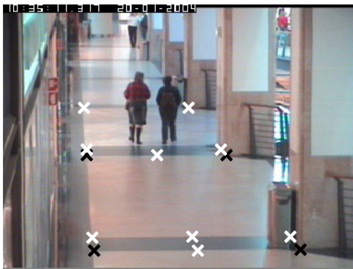
Figure 3.5: Image from [CAVIAR, 2004] with crosses from the camera calibration method
