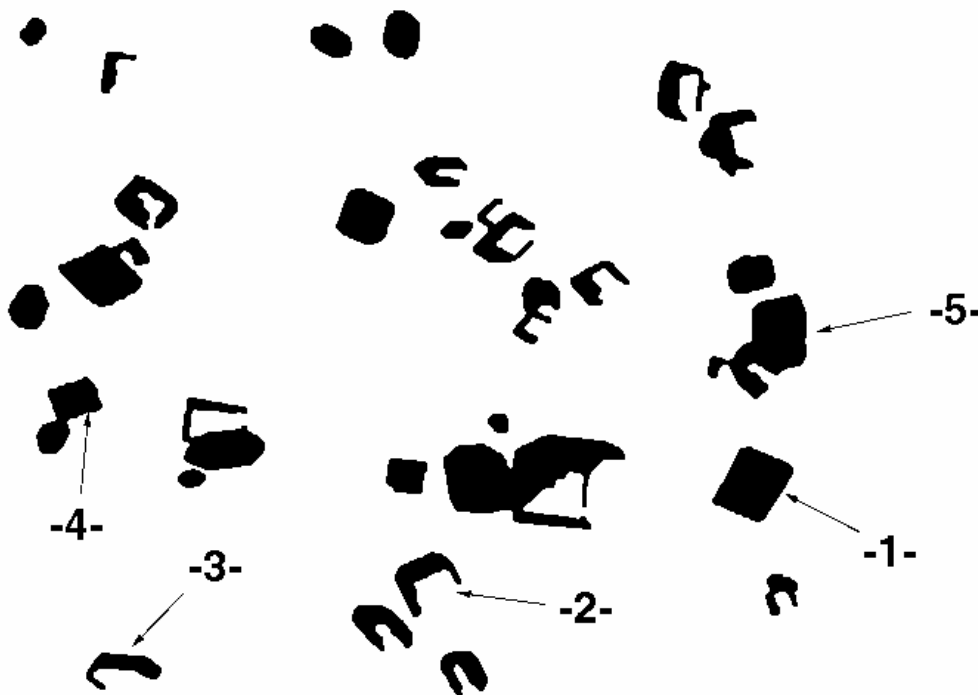
Figure 2.3. Identification of different types of silhouettes, from which, crystal equivalent diameters were calculated.
