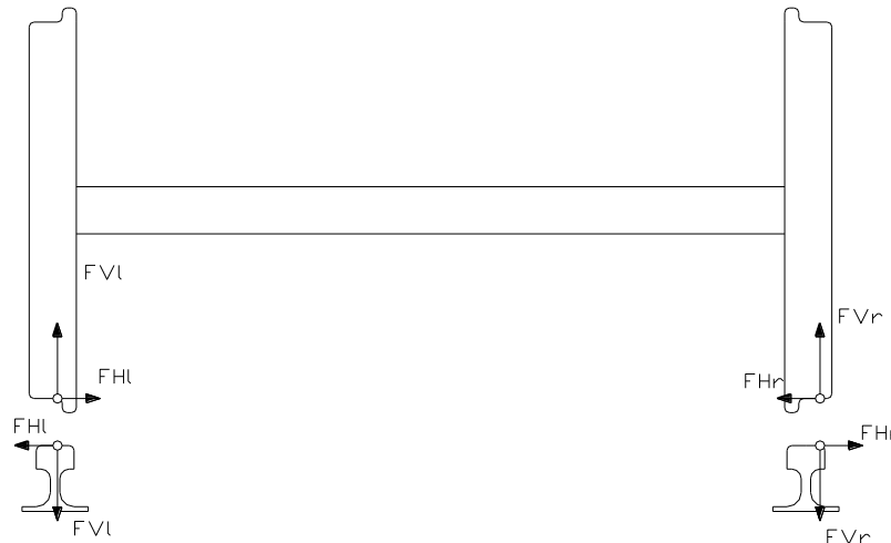
Figure 2.27 – Vertical and horizontal contact forces between wheel and rail, (Andersson et al., 2002)
