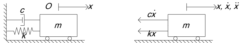
Figure 2.3 – Single DOF system with damping
