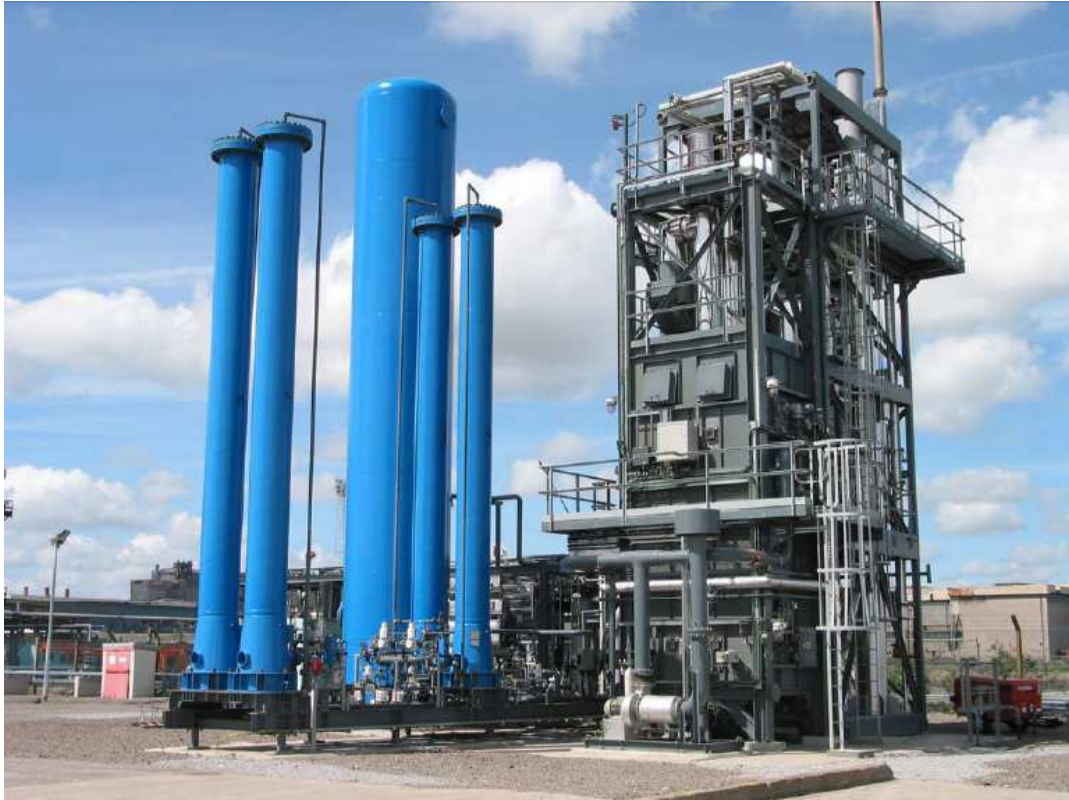
Figure 1.3 – A steam methane reforming (SMR) process for the hydrogen production ( 800 \text{ m}_N^3 \cdot \text{h}^{-1} ) (Allam, 2004).
