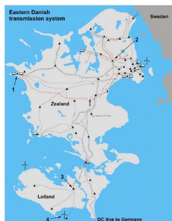
Figure 2.4 - DK-East transmission system. Source: “Phasor measurement of wind power plant operation in Eastern Denmark”, Joana Rasmussen & Arne Hejde Nielsen
