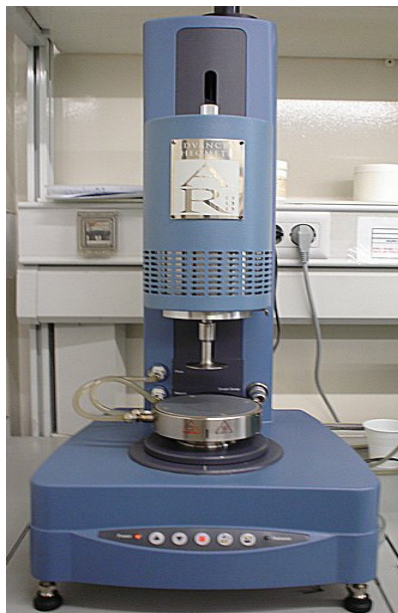
Figure 2.1 The controlled stress rheometer (TA instrument AR2000) fitted with the cone-and-plate geometry.
