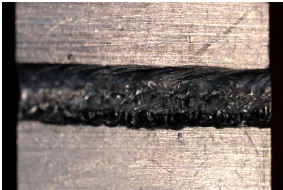
Fig. 55 - macrography of the specimen with welding defects - W2-F2
