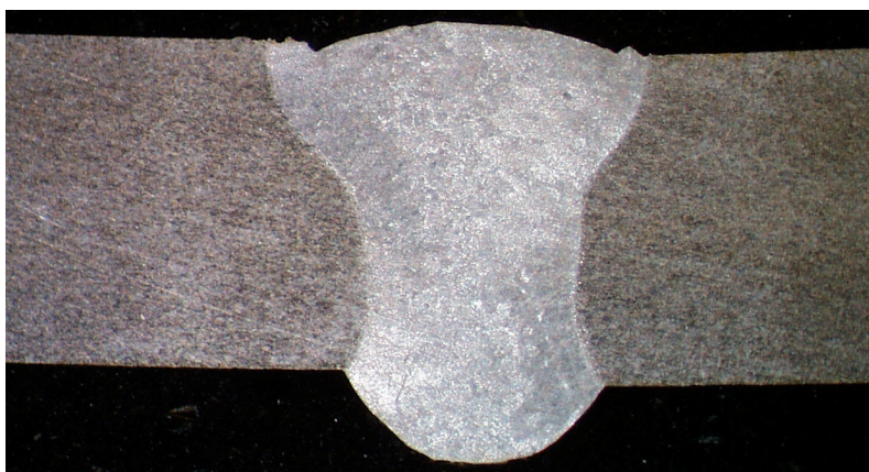
Fig. 50 - macrography of welding zone
