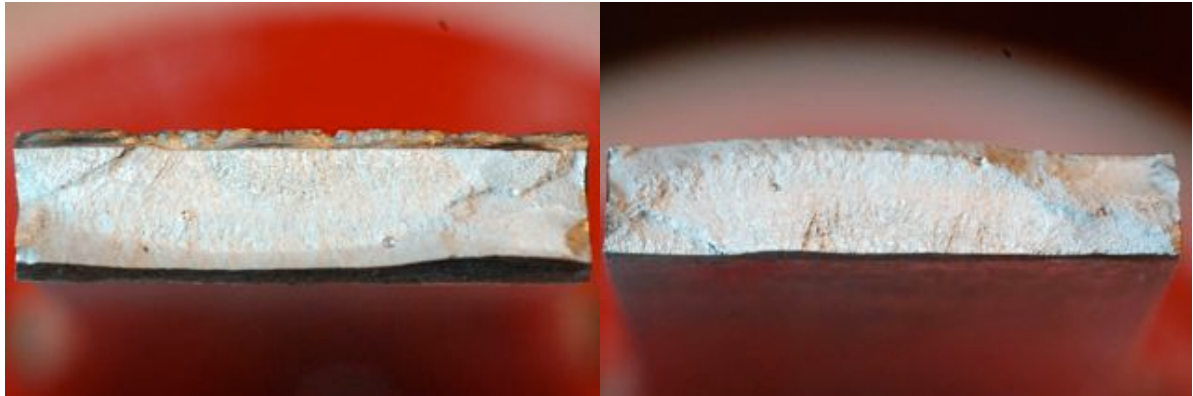
Fig. 54 a) - fracture surface of fatigue specimen W3-F2
