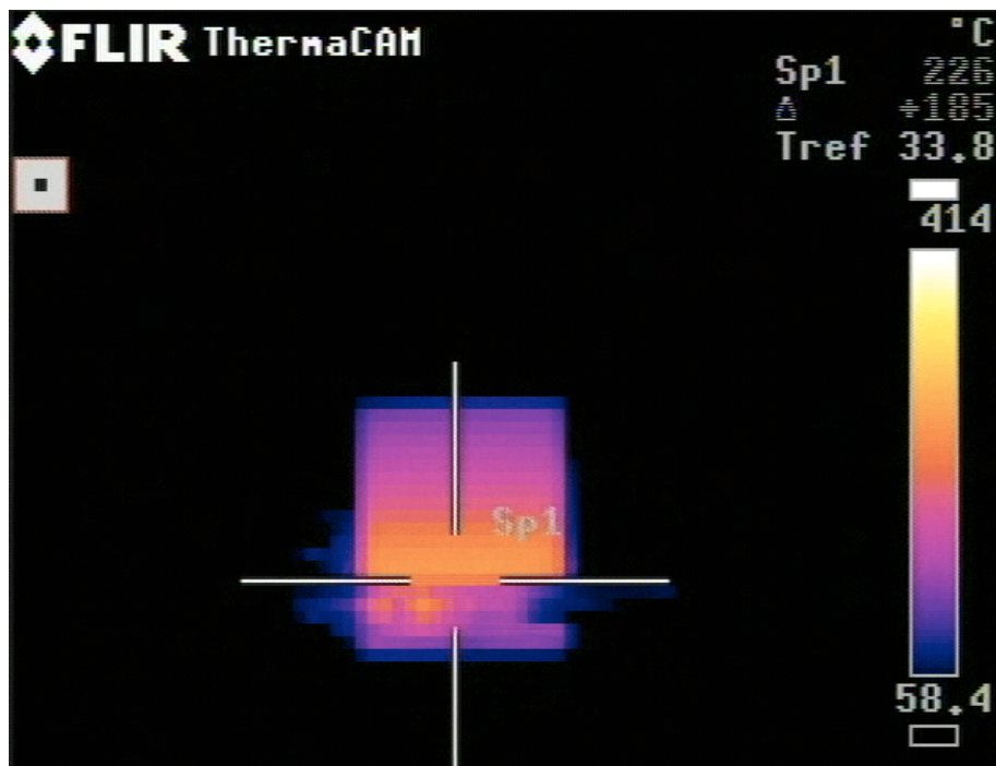
Fig. 8 b) - infrared thermography frames - FS tool, 20 seconds
