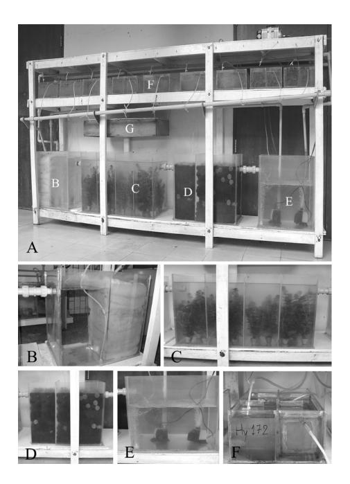
**Figure 3.2.** Photographs of the aquaculture system II used to rearing freshwater mussel juvenile (0-120 days old). Close recirculation system (A); Particulate filter cabinet (B); Macrophytes filter cabinet (C); Biological filter cabinet (D); Reservoir tank (E); Juvenile culture box (F); Fluorescent box (G).
