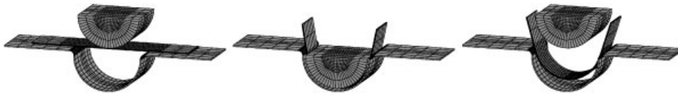
Figure 29. Main time steps in the cylindrical bending.
