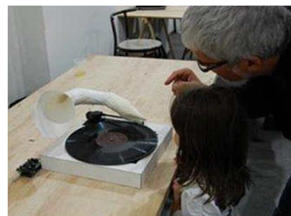
Figure 5. A climate data driven record player which adjusts its playing speed in reaction to data from a Timestream.
