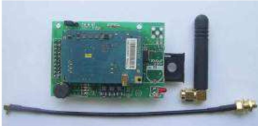
Figura 3.3. Transreceptor GSM – GR64
