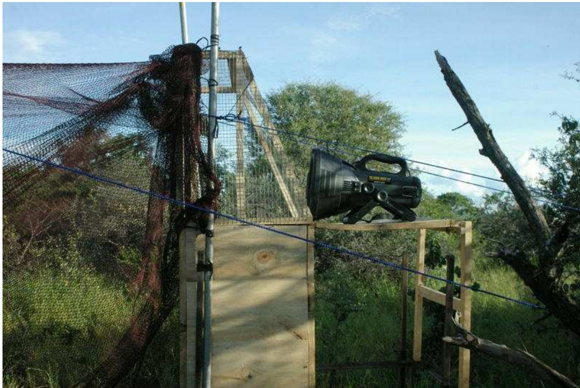
Plate 5.5. The Funnel trap, with a Heligoland trap style catching box, in the field with the floodlight in position (Photo: R. A. Cheke).
