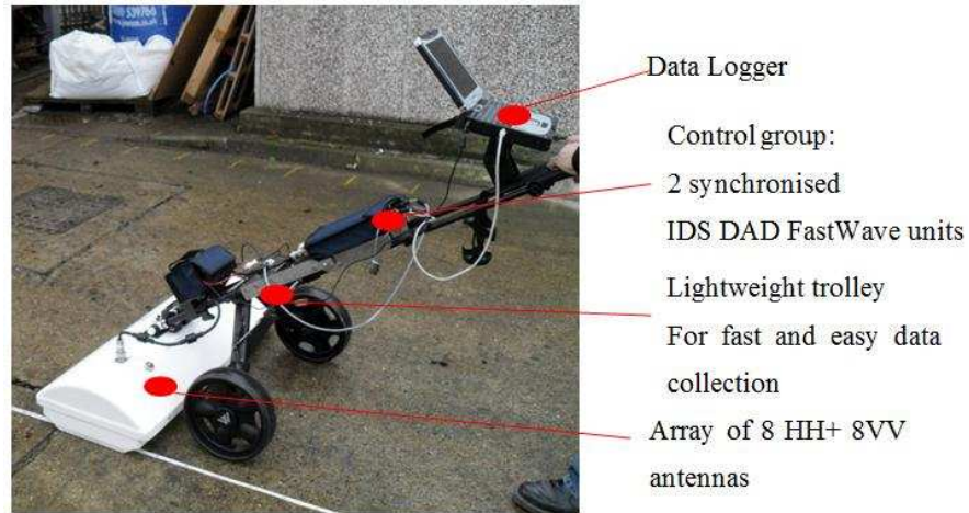
Figure 3.5 – GPR Hi BriT GPR Antenna (Photos from Gokhan Kilic, 2010)
