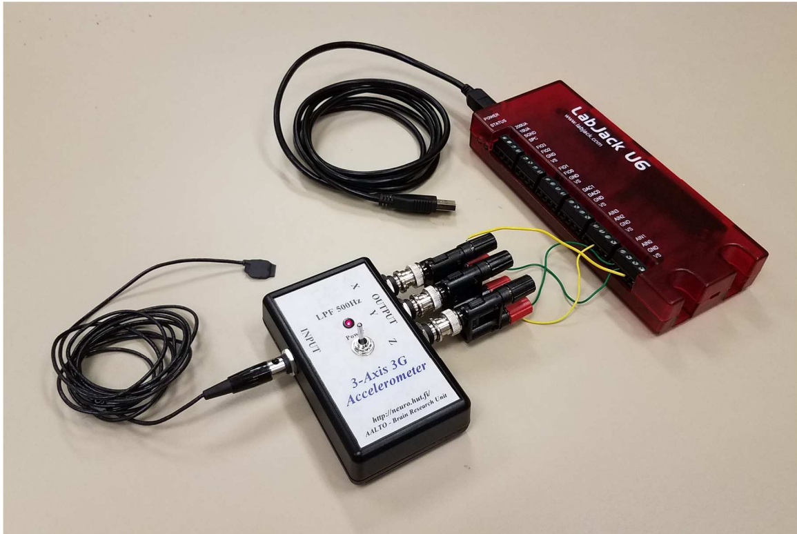
Figure 3-2: The three-axis accelerometer connected to the LabJack U6 USB DAQ device. The ADXL330 accelerometer (in black, on left) is connected to a unit (labeled “3-Axis 3G Accelerometer”) that filters signals to three separate BNC connector outputs. Each of the BNC outputs (X, Y, Z) has an adapter and single wire connected to one of the LabJack U6 DAQ (labeled, in red) analog inputs (AIN0, AIN1, AIN2). There is also one ground connection from the BNC output (X) to the DAQ ground input (GND). The DAQ connects to a computer via USB.
