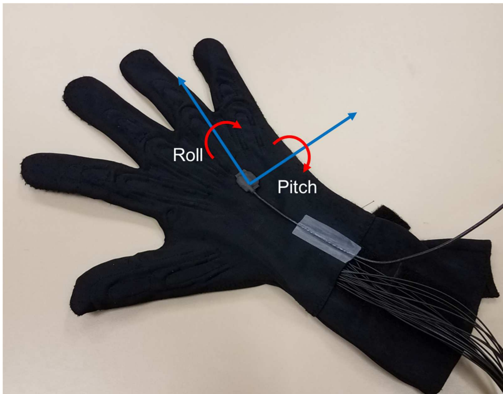
Figure 3-6: Axes along which the roll and pitch angles are measured on the glove and accelerometer. Although not shown here, the accelerometer was taped down to the glove on the back of the subject’s hand to prevent it from changing position. Roll angle corresponds to the rotating the wrist while pitch angle corresponds to tilting the hand forward or back.
