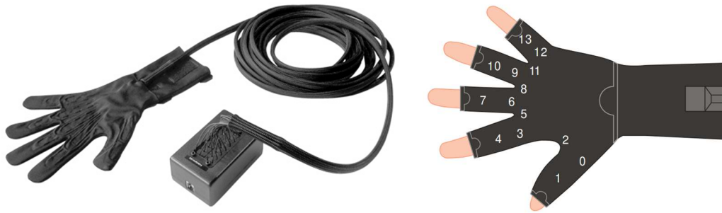
Figure 3-3. The 5DT Ultra 14 Data Gloves (right hand only pictured on left) has 14 optical sensors that are wired to a driver (black box on left). The driver connects to the computer via USB (not pictured). Each of the 14 optical sensors on the glove (right) are located at two joints on each finger and between each finger, along the back of the hand. (5dt.com)
