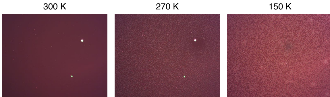
Figure 3.12: Particles form on sample as soon as it is cooled below room temperature. Chamber pressure was 5mTorr.
