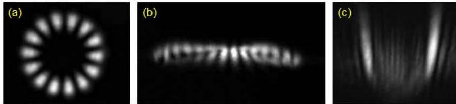
Figure 4-10: (a) Equal parts l = 7 and l = -7 launched into mode sorter from air core fiber (b) Transformed beam leaving sorter (c) Transformed beam focused by cylindrical lens, yielding spindle-like patterns, one for each l
