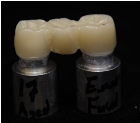
Figure 92: Sample# 7 (YZ-e.max fused aged)
