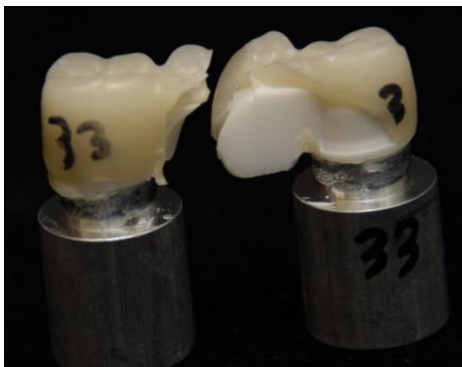
Figure 109: Sample# 33 (YZ-Triluxe cemented aged)
