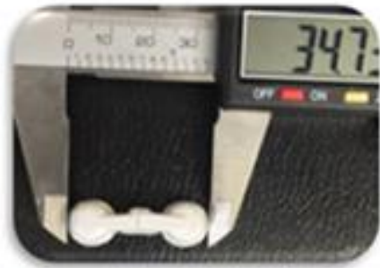
Figure 13: Milled Zirconia Frame Before Sintering
