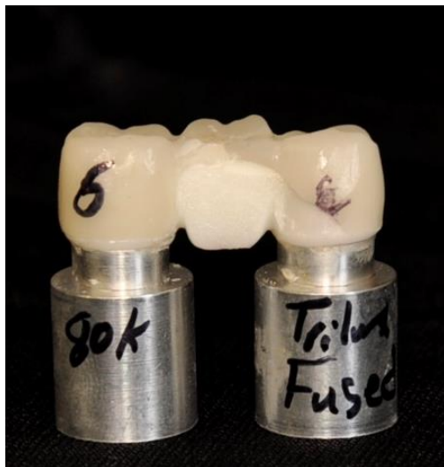
Figure 67: Sample# 6 (YZ-Triluxe fused 80K)
