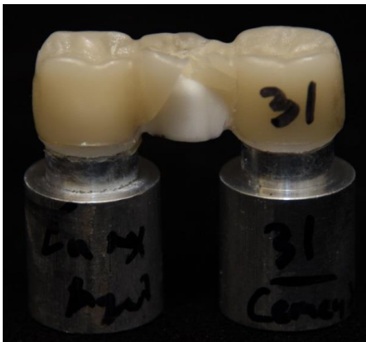
Figure 107: Sample# 31 (YZ-Triluxe cemented aged)
