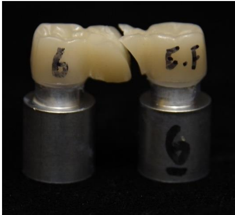
Figure 91: Sample# 6 (YZ-e.max fused aged)
