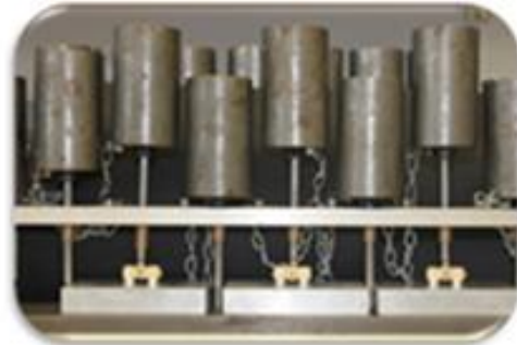
Figure 21: Cemented bridges under loading apparatus
