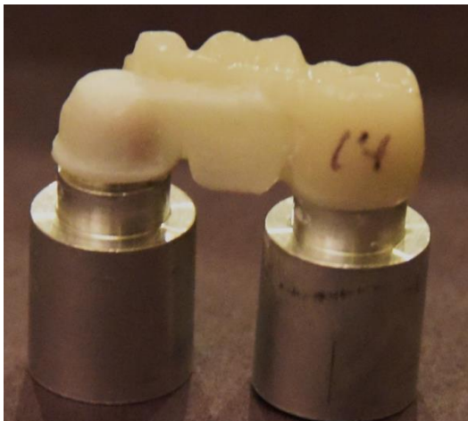
Figure 46: Sample# 14 (YZ-Triluxe fused)
