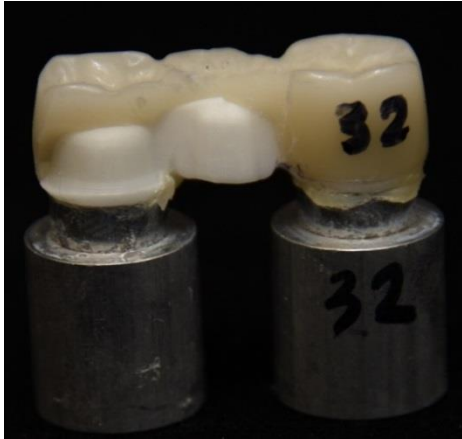
Figure 108: Sample# 32 (YZ-Triluxe cemented aged)
