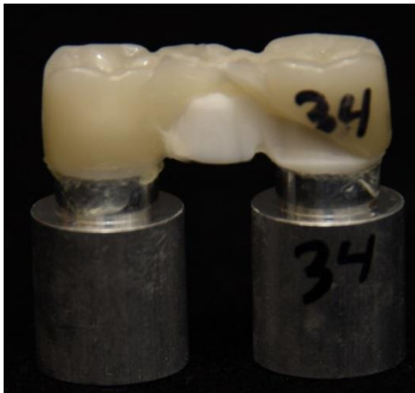
Figure 110: Sample# 34 (YZ-Triluxe cemented aged)
