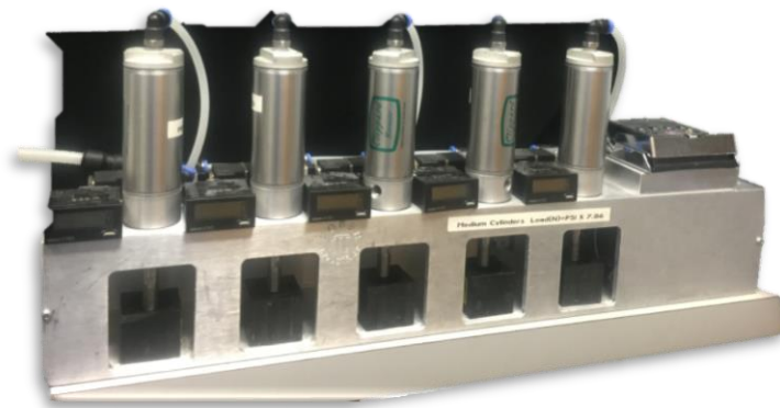
Figure 30: Cyclic loading apparatus, Pober Industries, Waban MA
