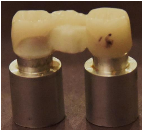
Figure 47: Sample# 16 (YZ-Triluxe fused)
