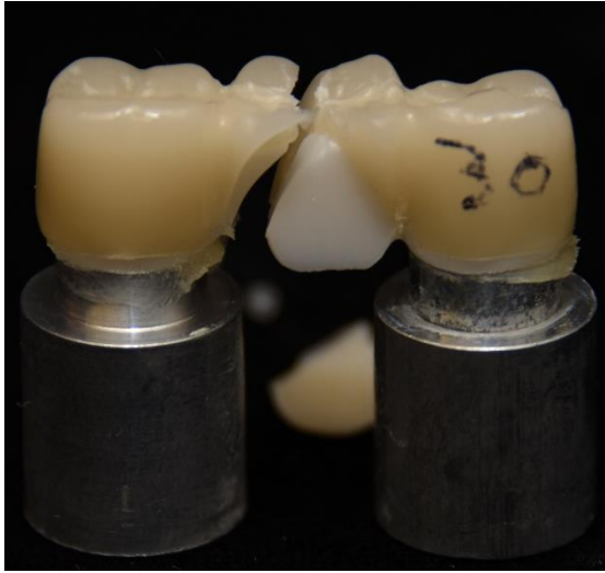
Figure 106: Sample# 30 (YZ-Triluxe cemented aged)
