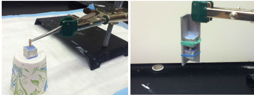
Figure 12. Potting of Superior and Inferior Ends of Femur. Figures taken from A. Wulff, 2015.
