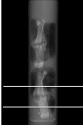
Figure 8. Scout View of Micro-CT Image. Two femurs stacked vertically. The two horizontal lines on the bottom femur are the start and stop points for the scanner. The area in this image is the area taken up by the fracture callus. In non-fractured femora the region was uniformly distributed into 309 slices, equivalent to 3.7 mm at the mid-diaphysis. Figure taken from A. Wulff, 2015.
