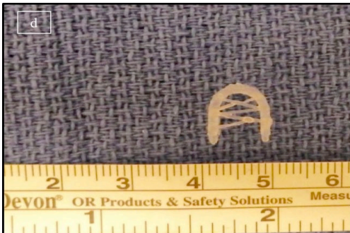
Figure 5d): Pluronic® F12 “U” shaped macrochannel melt fused to manually extruded Pluronic® F127 to form the macro and microchannel network.
