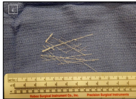
Figure 5c: Manually extruded Pluronic® F127 will be sacrificed in type-I collagen to create the microchannels.
