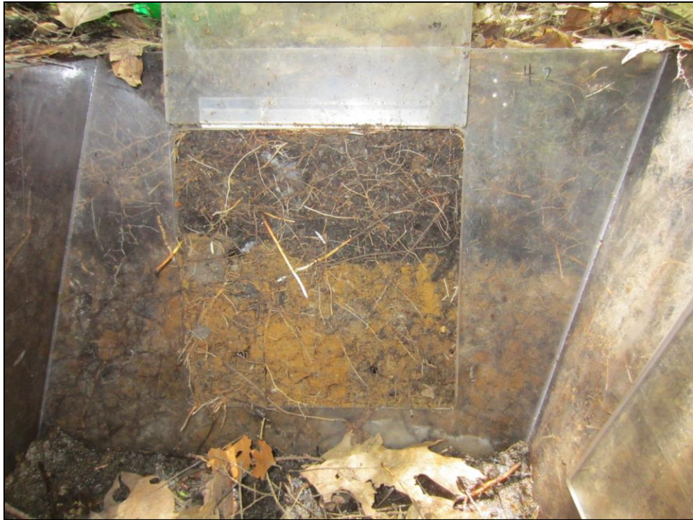
Figure 4.1. Plexiglass root box designed and constructed for this study at Boston University. Roots can be accessed by lifting a hinged panel. The second hinged panel is partially visible in the lower right hand corner.
