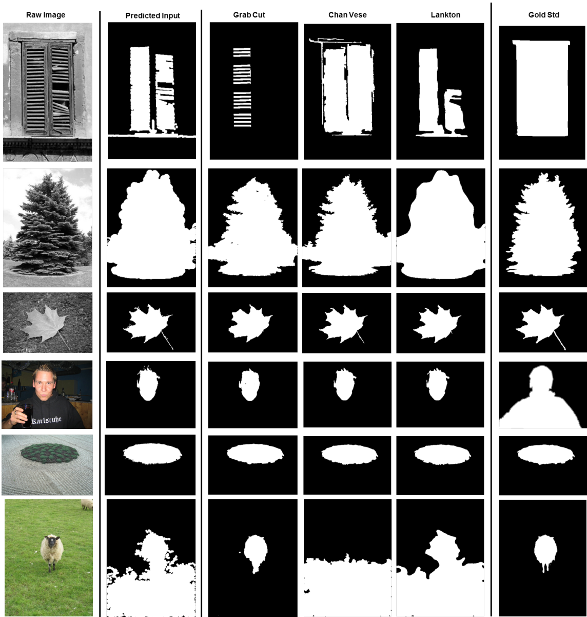
Figure 7.5: Sample results for the everyday images (i.e., Weizmann and IIS). See the previous figure for the explanation of the image layout. In some cases, an interactive segmentation algorithm can perform well when using a low quality segmentation as input, as observed for the image of the sheep (row 6, Grab Cut algorithm). In other cases, none of the interactive segmentation algorithms perform well when initialized with a low quality segmentation, as observed for the image of the person (row 4).
