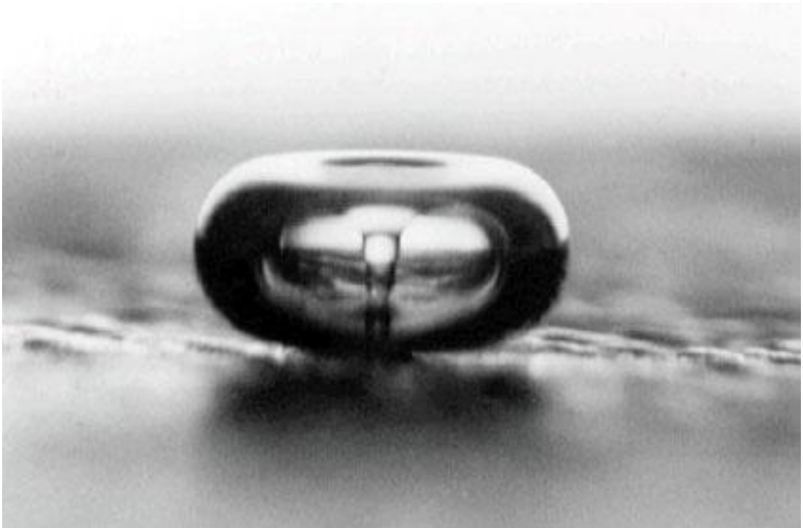
Figure 1.4: A bubble implodes near a solid surface. The presence of the solid causes the collapse to be asymmetrical, forming a high-speed jet of liquid that impacts the surface. (from L. A. Crum, Ph.D., University of Washington, Applied Physics Laboratory). Bubble diameter approximately 1mm
