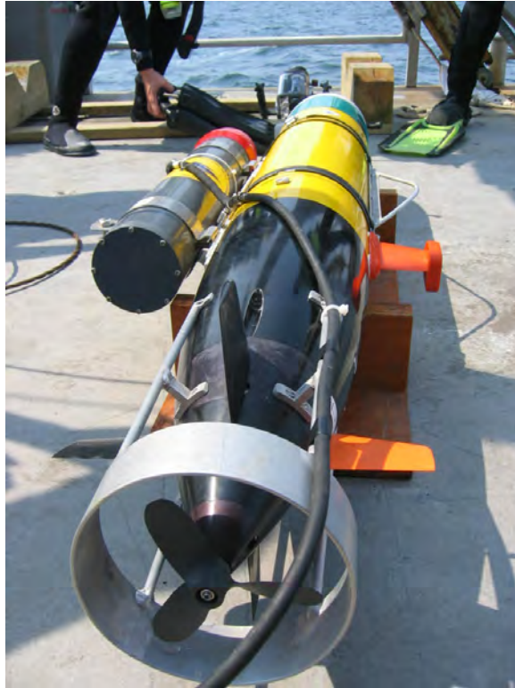
Figure 3.14: Photograph of the vehicle with a more stable array attachment. The vehicle is on its side in its cradle with the top to the right. The lifting bail, recording canister, and shroud are clearly seen.
