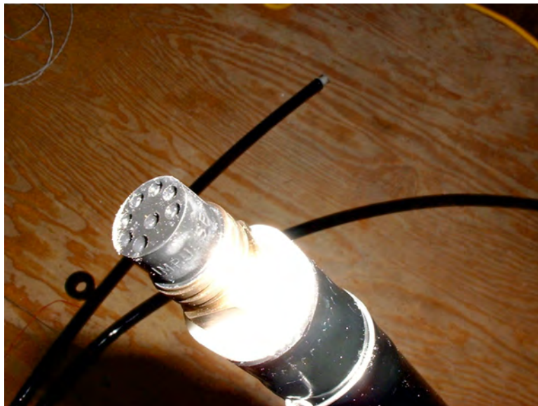
Figure D.7: Photograph of the connector, termination, and wire clamp on the front of the acoustic section of the array
