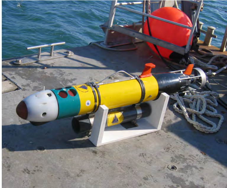
Figure D.2: Photograph of the REMUS 100 AUV used in the experiments. Here the vehicle rests on the deck of R/V Tioga in its cradle. The propellor shroud, recording canister, and lifting bail are all clearly visible.
