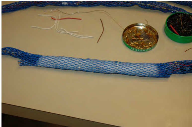
Figure D.5: Photograph of hydrophone group wrapped in batting material and inserted in the mesh sleeve
