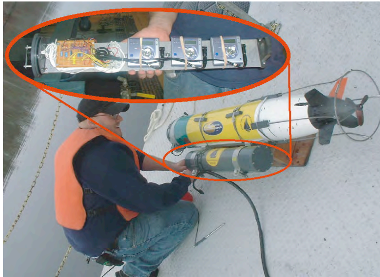
Figure D.14: Photograph of recording system including its location when strapped to the AUV
