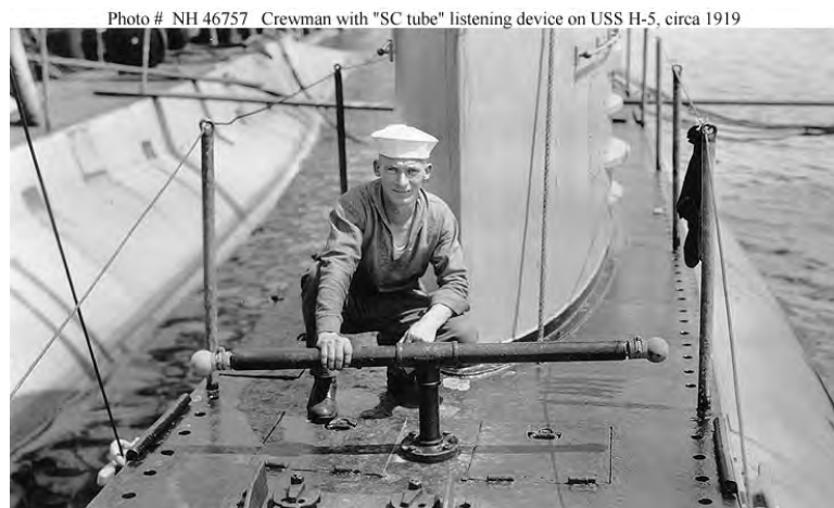
Figure 1.1: A crewman of the USS H-5 seen with an early sonar listening device.[3] The use of two transducers on a rotating shaft provided directionality and was perhaps the first major advance in sonar technology since Da Vinci.
