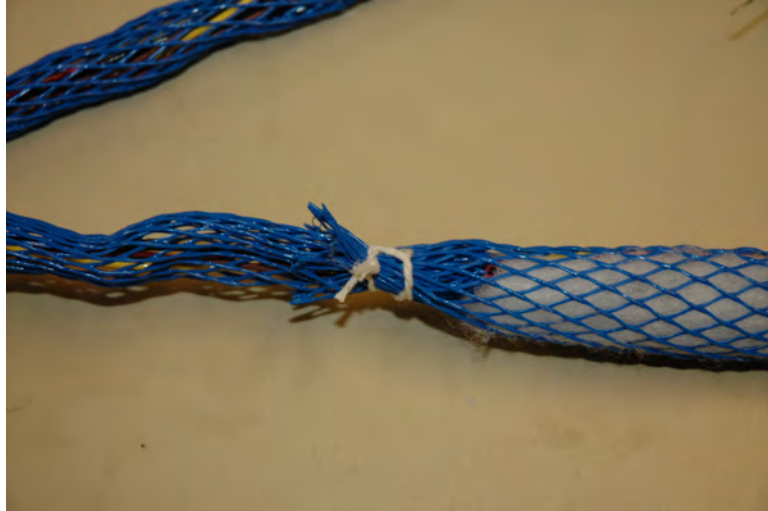
Figure D.6: Photograph of a tie off used on the mesh sleeve to keep array components in place
