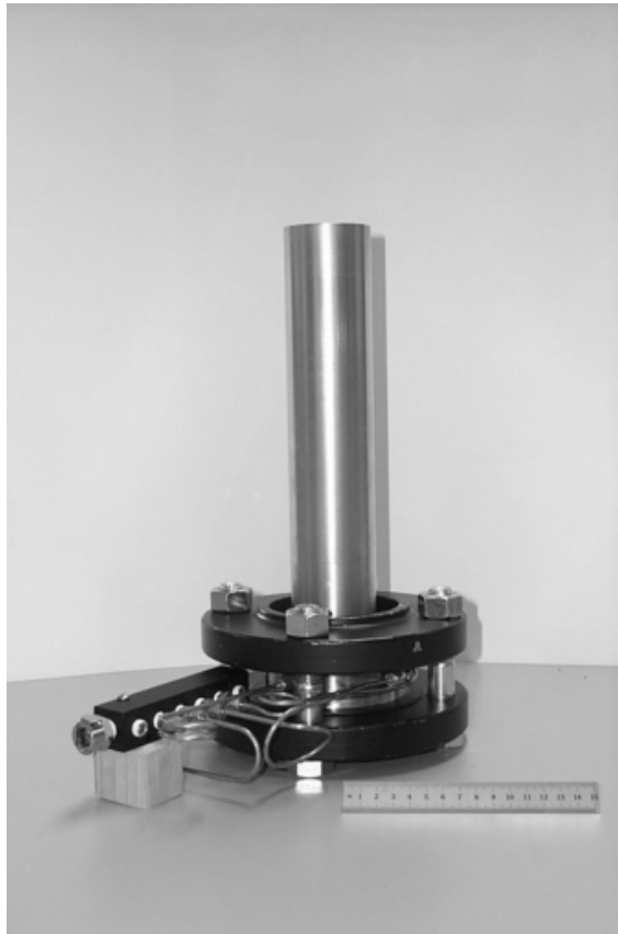
Figure 4.9: A photograph is shown of the void fraction resonator with the bubble injection manifold mounted at the bottom of the tube. The scale is 15 cm in length.
