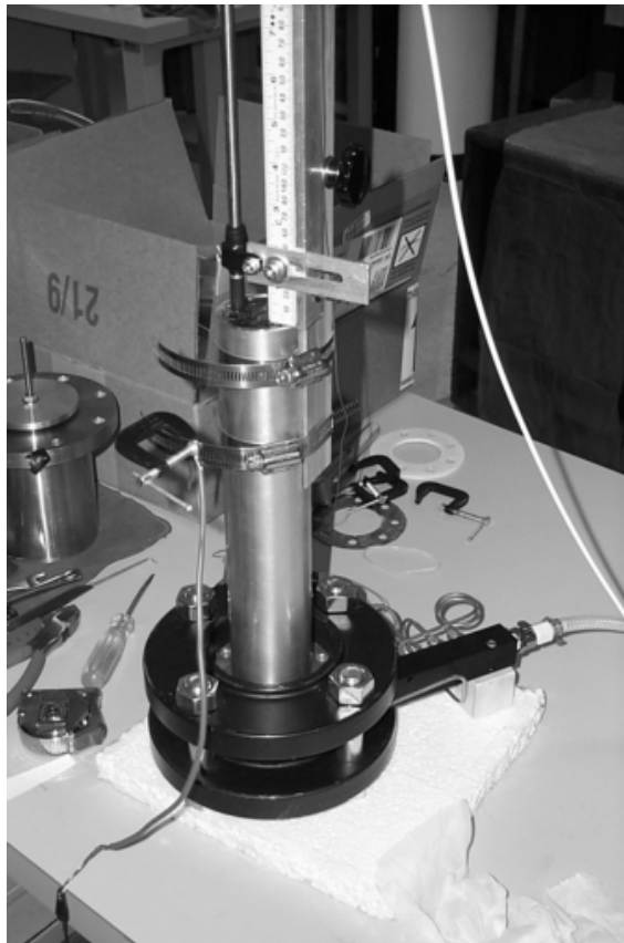
Figure 4.10: The void fraction resonator is shown with the hydrophone positioning system attached.
